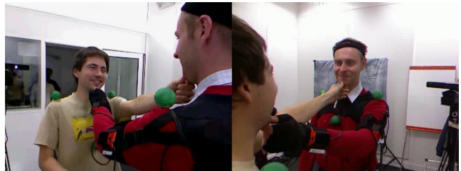
Figure 1: A frame from MMLI recordings [15]. On the left: a participant is wearing green markers. On the right: another participant is wearing a motion capture suit and green markers.
