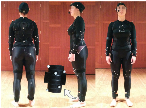
Figure 4: Markers and rigid bodies placed on the dancer’s body. A rigid body is a rigid plate on which several markers are attached. This configuration allows us to extract not only the position but also the rotation of body joints. In the figure, the lower left leg rigid body is highlighted.
